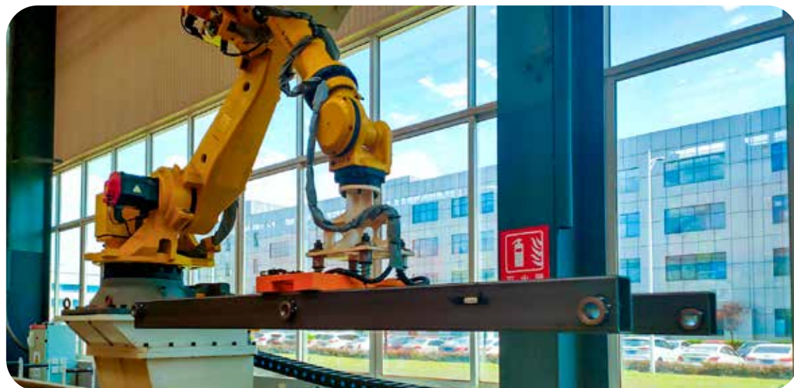
Pick and place of structural steel (H beam blanks, angle iron, square tubes, pipes etc.)
