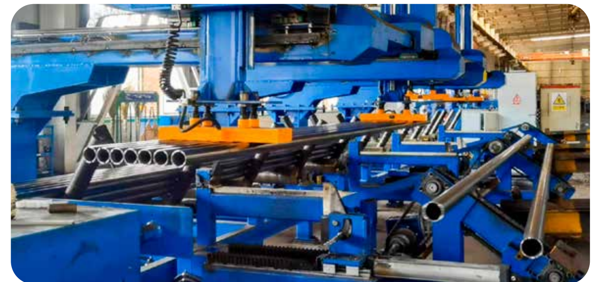
Pick and place of structural steel (H beam blanks, angle iron, square tubes, pipes etc.)
